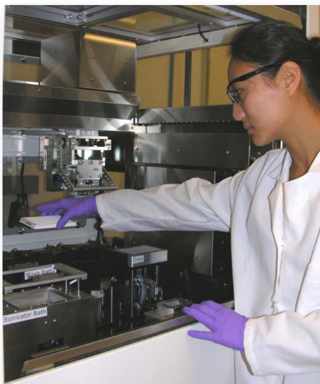
Catherine Chen, Ph.D., a biologist in the Therapeutics for Rare and Neglected Diseases program, loads a microplate containing cells that model a rare disease onto the pintool machine to allow high-throughput screening of small molecules.
